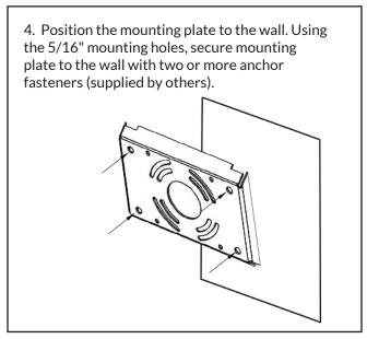
NOTE: Techlight recommends securing to both the J-Box and wall for additional support. Use anchors or screw hardware appropriate for building wall substrate (supplied by others).
