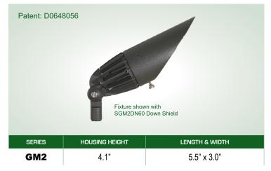
**MOUNTING** — The die cast aluminum mount is secured to the heat sink by stainless steel screws and is sealed with an integral o-ring. A 1/2" threaded knuckle is provided standard.
