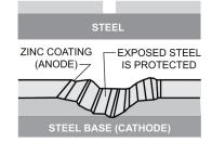
**Galvanized Steel** This is what happens at a scratch on galvanized steel. The zinc coating sacrifices itself slowly by galvanic action to protect the base steel. This sacrificial action continues as long as any zinc remains in the immediate area.
