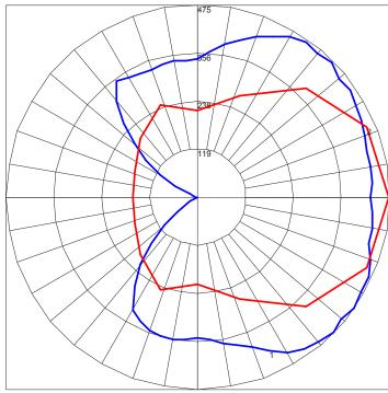
$\label{eq:maximum Candela = 475} \begin{array}{ll} \text{Maximum Candela = 475} & \text{Located At Horizontal Angle = 0, Vertical Angle = 45} \\ \text{\# 1 - Vertical Plane Through Horizontal Angles (0 - 180) (Through Max. Cd.)} \\ \text{\# 2 - Horizontal Cone Through Vertical Angle (45) (Through Max. Cd.)} \\ \end{array}$
