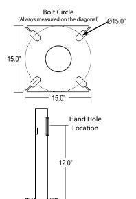
(2 Piece Pole) 45' Steel Round Tapered 7 Gauge Pole
