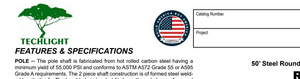
ed longitudinally. The hand hole is located 1' above the pole base. A ground lug is provided standard. These poles are 2 piece poles and are shipped as such. Field assembly required.
