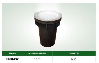
**MOUNTING** — Fixtures are designed to be in-ground burial lights and should be installed according to the installation instructions made available by Techlight. Proper drainage and substrate must be provided for water to flow freely through the well sleeve. A  $\frac{3}{4}$  conduit entry is supplied into the anti-siphon chamber of the housing. Conrete pour kits available (see Accessories).
