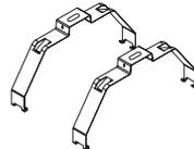
Securely attach mounting brackets (2) to mounting surface. The enclosure will engage the mounting brackets at any point along its length except for where there are latches. It is recommended that the dimension between brackets equal about 60% of the fixture's length.
