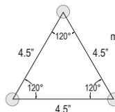
Bolt Pattern measures 4.5" bolt to bolt.
