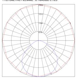
$\label{eq:maximum Candela = 23081.95 Located At Horizontal Angle = 60, Vertical Angle = 4 $\# 1 - Vertical Plane Through Horizontal Angles (60 - 240) (Through Max. Cd.) $\# 2 - Horizontal Cone Through Vertical Angle (4) (Through Max. Cd.)}$
